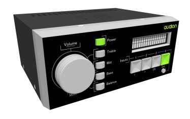
Thank you for you purchase of the qtone DA-1001 20W Digital Amplifier. The unit has 4 inputs as well as 2 outputs and up to 20 watts of amplification. As a digital amplifier it is very efficient (up to 93%!) While no audio is provided the amplifier uses very little power and while in use, due to its efficiency, requires no heat-sink.
